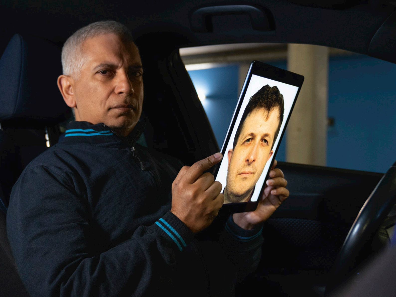
An Idiap staff member testing whether a facial recognition system can reject attempts at fraudulent identification.
