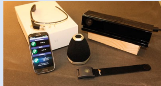
Figure 10 Sensors available in the social sensing lab. Kinect V2, Microcone, Q-Sensor, Android smartphone, Google Glass.
