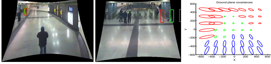
Figure 2: Left images. Due to depth effects, very similar positions in the first camera view corresponds to dramatically different image locations on the other view. Right graph. for the same scene, floor map of localization uncertainties, propagated from image localization uncertainties. In green, floor locations visible in both cameras. In blue/red, locations visible by only one camera.
