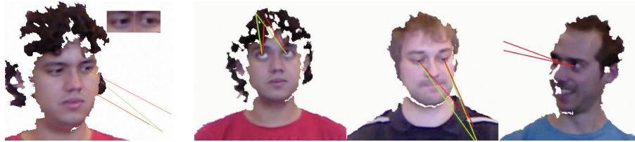
Figure 12.4 Left: 3D rendered mesh from depth and RGB image. Left top: using the 3D tracker output, eye regions from the RGB image can be cropped and rendered as if the head pose was frontal. Right: example of recognized gaze for different individuals under free head movements. Green lines (when available) materialize the ground-truth gaze directions, while the red ones represent estimated gaze.
