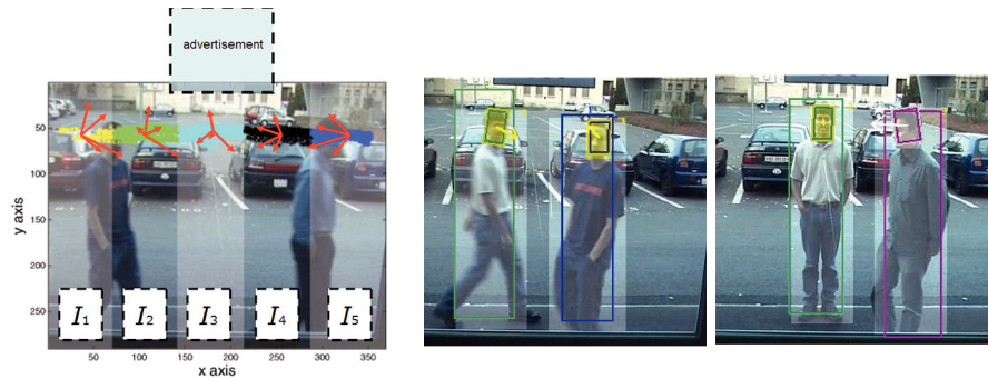
Figure 12.3 Left: wandering focus of attention (WFOA) modeling for the poster setup. The goal is to identify people looking at the advertisement. Head pose pointing vectors (red arrows) associated with looking at the poster are shown in each of the discrete space region. Right: sample results. White and yellow heads indicate a person recognized as looking or not at the poster.
