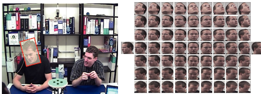
Figure 12.1 Head pose extraction. The head localization (position, scale, in-plane rotation, in the left image) and head pose (discrete index identifying a specific out-of-plane rotation, in the right image) are jointly tracked.
