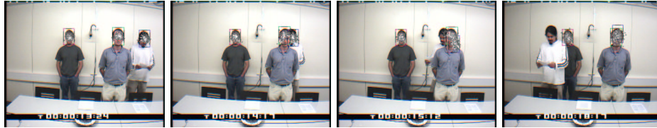
Figure 9: Tracking results for RealSeq2 . PS (1 → 2 → 3) fails to recover from occlusion (frames 2,20,40,120 shown) success and recovery rate: 8%. Particle ( u, v ) positions are superimposed on the image. Brighter pixels indicate higher likelihoods (139 frames at 360x288). On the contrary, DPS has higher success and recovery rates: 60% and 88% respectively.
